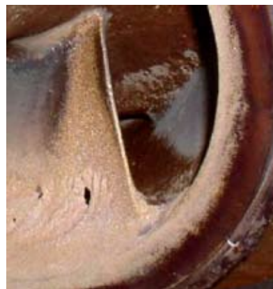
Fig. 1.5: Impeller showing cavitation damage (Source: KSB Centrifugal Pump Lexicon)
