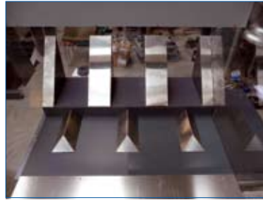
Fig. 5.4a: Model for a waste water pumping station with benching and bottom flow splitters
