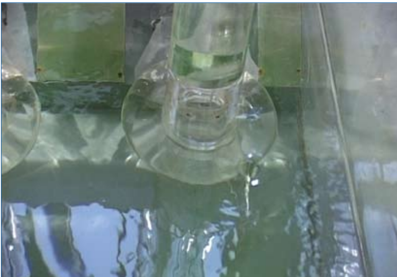
Fig. 5.1: Air-entraining vortex at a model pump
