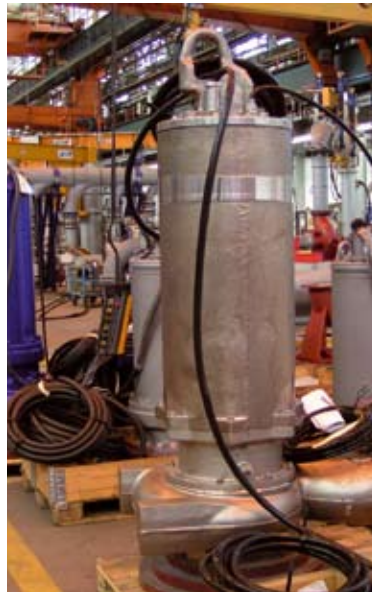
Fig. 2.4: KRT for seawater applications, completely made of duplex stainless steel
