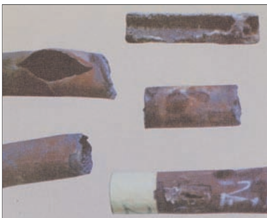
Photo 2.10 Bursting of superheater tubes by carryover
