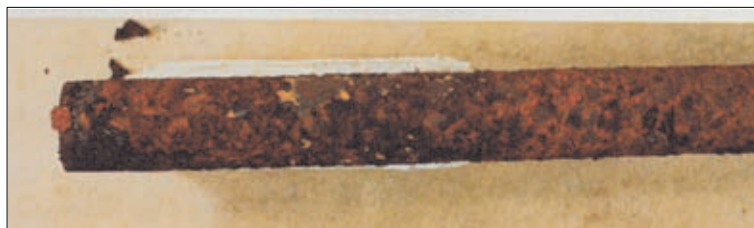
(b) Treated with an insufficient dosage of sodium sulfite against dissolved oxygen
