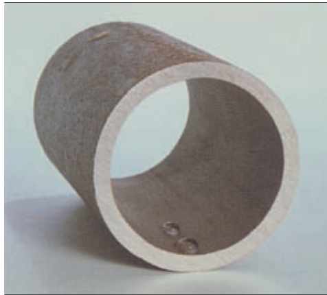
Photo 2.28 Water repellent condition on the protective film formed by a filming amine
