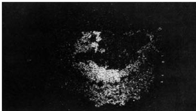
b) Chloride distribution in the pit by XMA inspection
