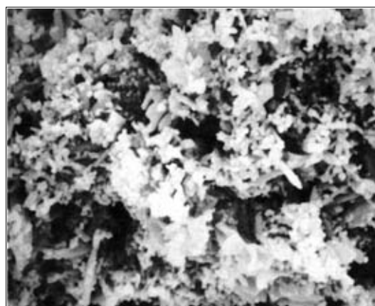
(Secondary electron image x 10,000) Photo 2.24 Particles of magnetite (without polymer dispersant)
