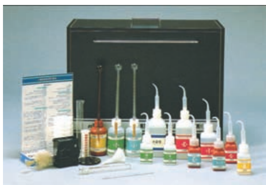
Photo 11.3 Water analysis kit for boiler and cooling waters
