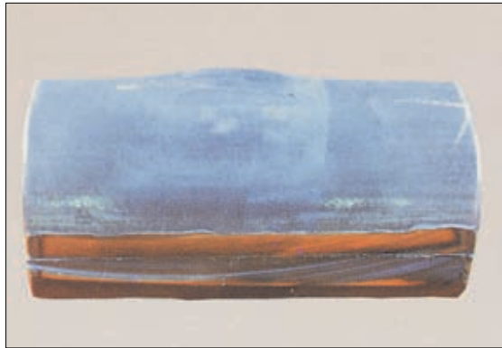
Photo 2.1 Expansion of an evaporation tube by scaling and overheating
