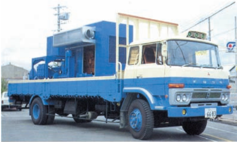
Photo 9.5 Mobile high pressure water jet cleaning system
