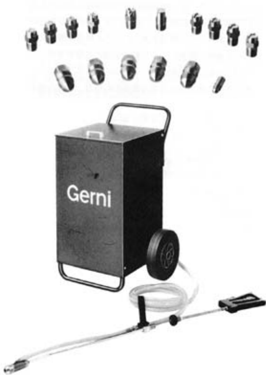
Photo 9.8 Wet sand jet cleaning apparatus and its nozzles
