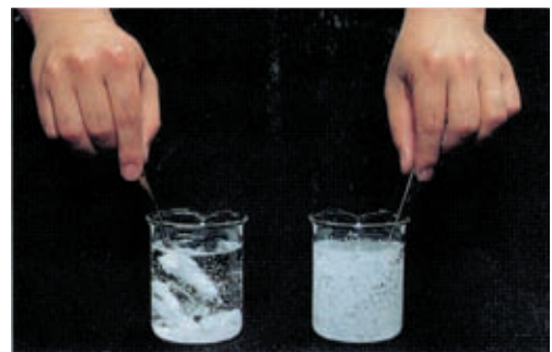
b) Dispersing condition of EDP FLOC Left: conventional flocculant Right: EDP FLOC
