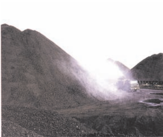
Photo 8.1 Sprinkling of a dust blow-away preventive using a sprinkling car
