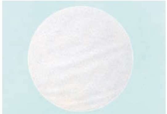
Photo 10.13 RO membrane after cleaning
