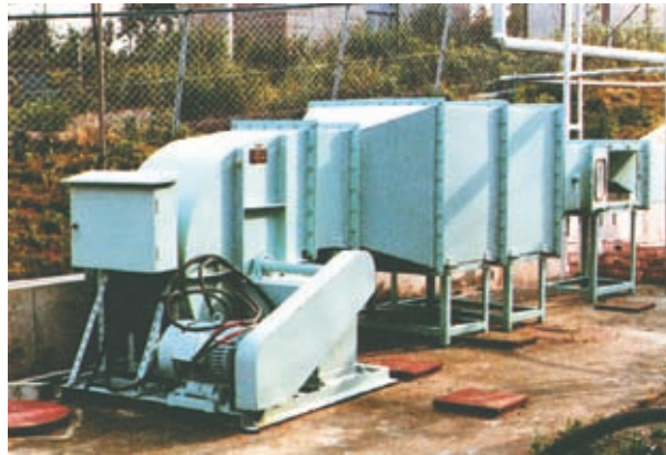
Photo 10.21 A wind tunnel for evaluating the effects of dust blow-away preventives
