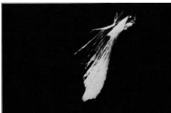
b) Changed crystal form of calcium carbonate by a scale inhibitor (x 7000 electron microscopic photograph)
