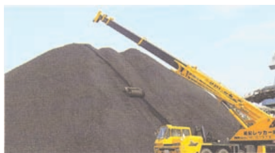
Photo 8.2 Surface conditioning of a coal pile by using a crane truck
