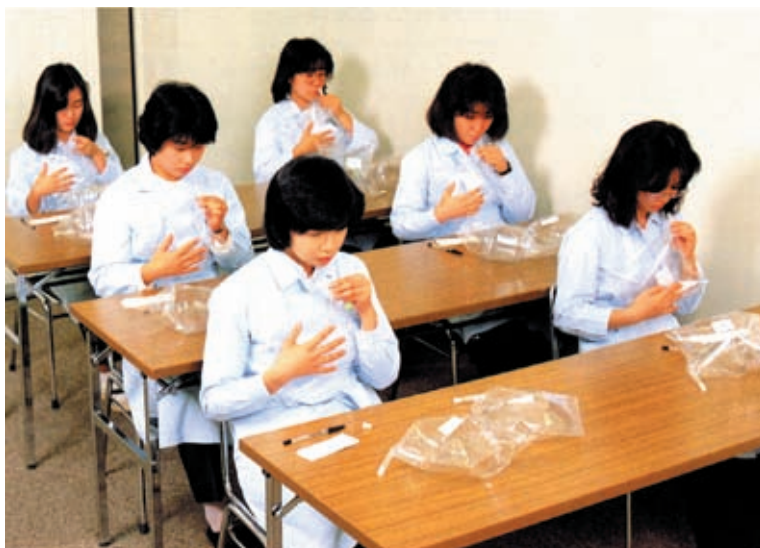
Photo 10.10 A view of the smelling bag method test for measuring the strength of an odor
