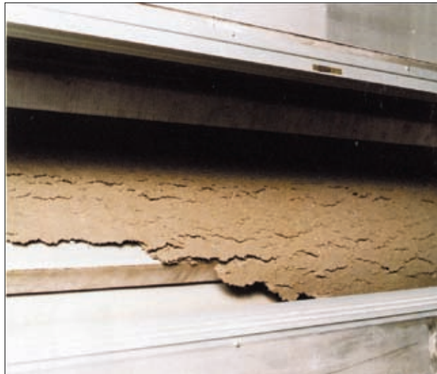
b) Dewatered cake of pellet type flocs and the removal condition from the filter cloth of a belt press dehydrator
