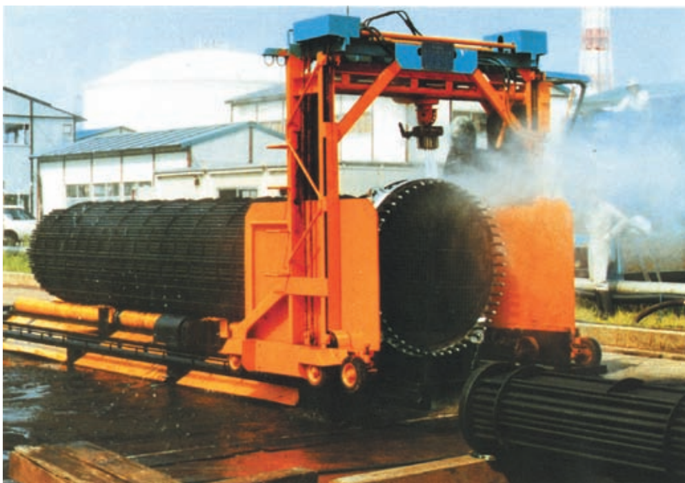
Photo 9.7 Automatic high pressure water jet cleaning system for the tube bundle of heat exchanger
