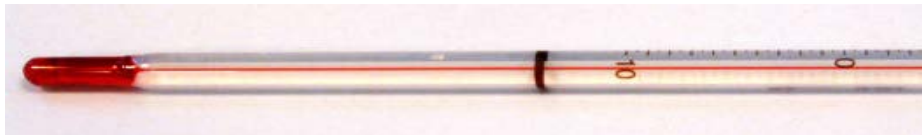
Picture of alcohol thermometer taken by chemical engineer from Wikipedia at http://en.wikipedia.org/wiki/File:SpiritTherm02.jpg
