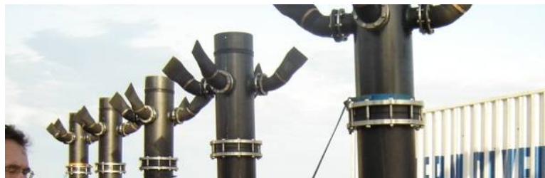
Figure 6-3. A rosette multiport brine diffuser.
