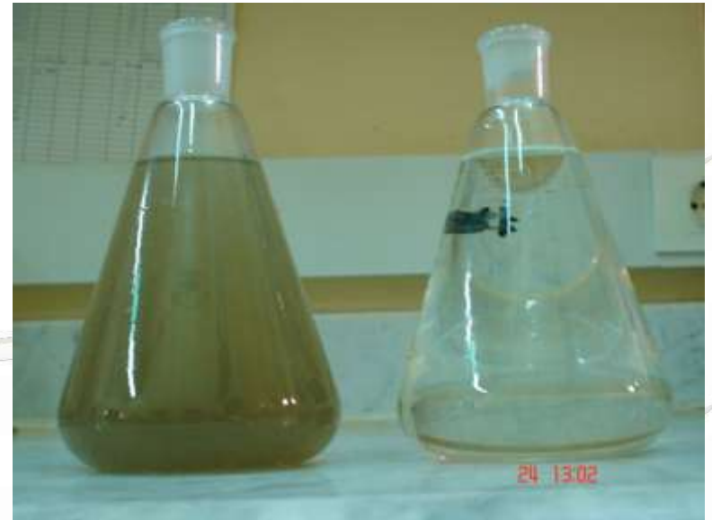
Domestic (Accommodation) Influent and Effluent from Almarai STP MBR.
