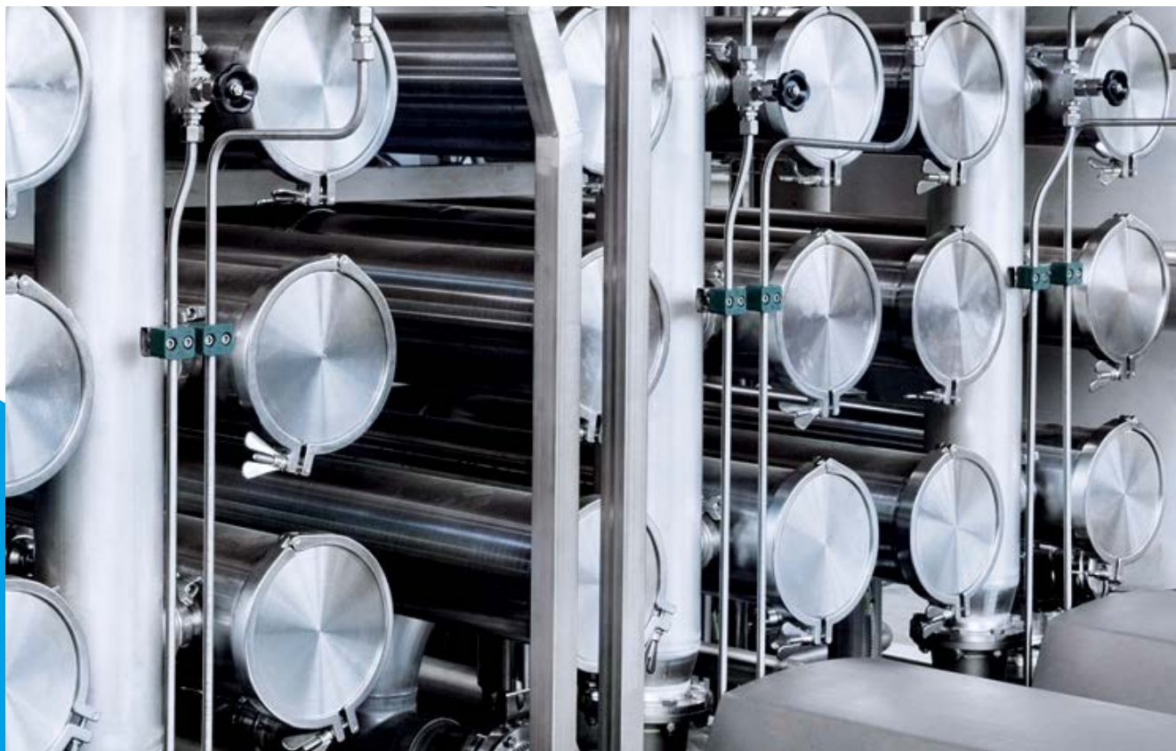
Nanofiltration is a cost-effective technology for partial demineralization of whey.
