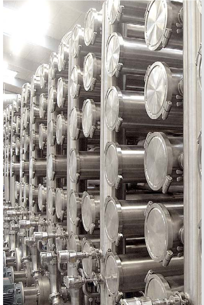
The ultrafiltration technology provides increased flexibility and yield in cheese processing.
