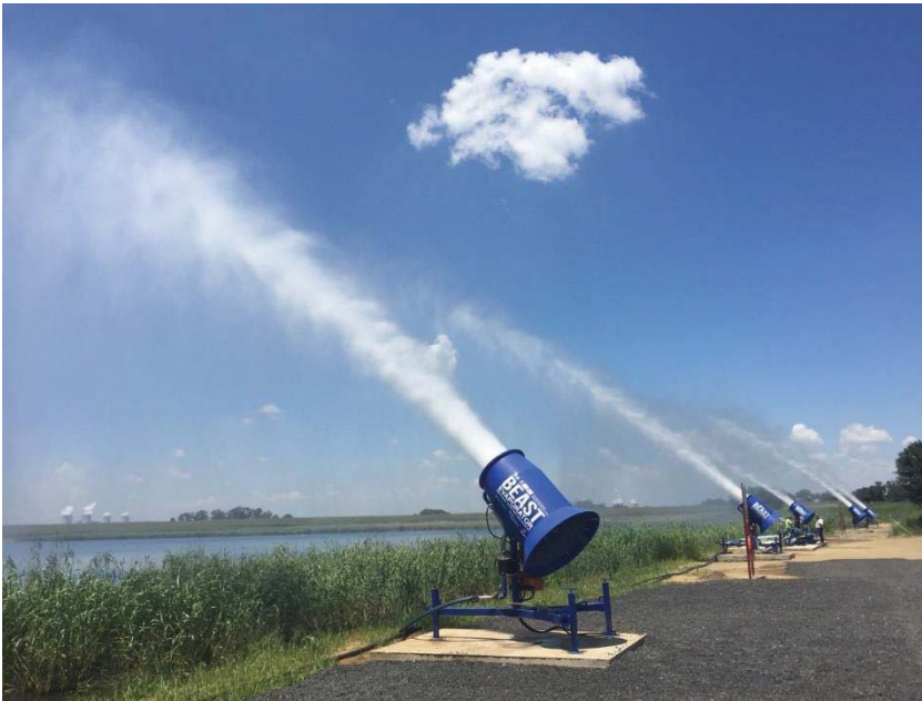
Figure 36: Mechanical evaporator equipped with a booster pump
