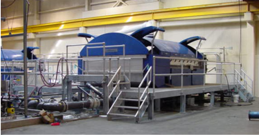
Gravity belt thickeners are often used to remove excess water from sludge.
