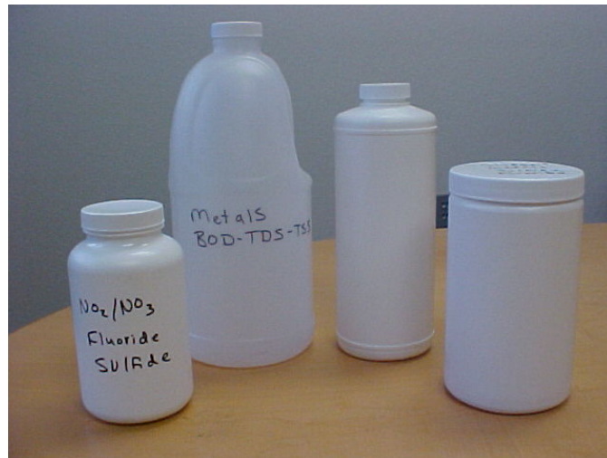
\text{NO}_2/\text{NO}_3 , Fluoride, Sulfide, Metals, BOD-TDS-TSS Wide-mouth Sludge/Metals bottle.
