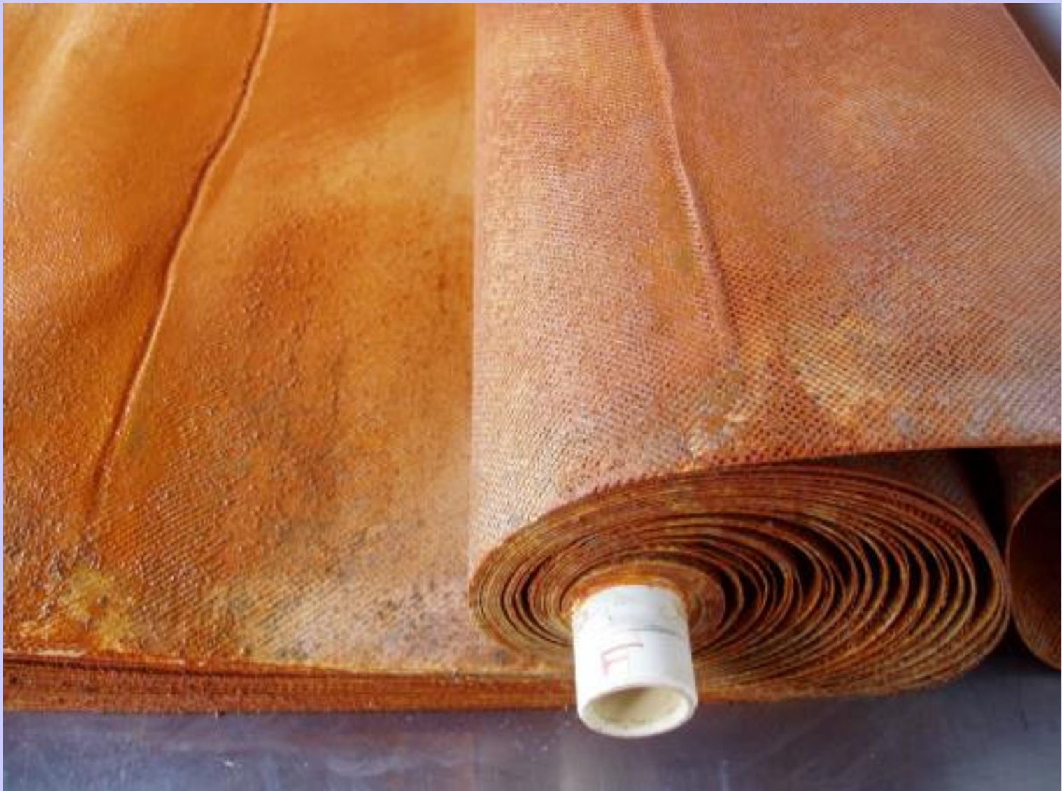
un-rolled feed-end. Note the heavy accumulation of foulant and depressions in the membrane leaf caused by foulant and pressure
