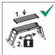
Secure the decking before use
