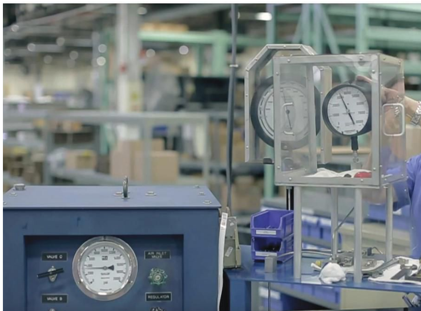
IMAGE 1: Pressure gauges being calibrated (Image courtesy of Ashcroft)
