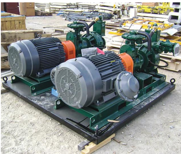
IMAGE 2: Skid-mounted system for oil and gas plant
