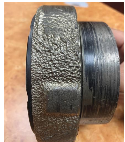
IMAGE 5: Signs of chemical attack (corrosion) in the front nondestructive evaluation (NDE) titanium bush housing assembly
