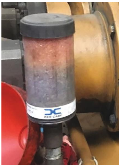
IMAGE 6: The direction of color change from top to bottom indicates internal water is present.
