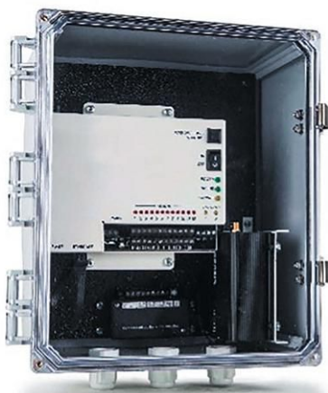
IMAGE 2: Remote monitoring base unit in a protective enclosure
