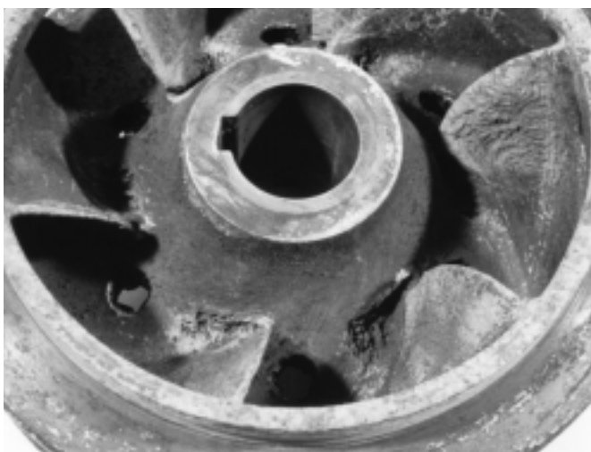
Fig. 6: Cavitation in bronze impeller
