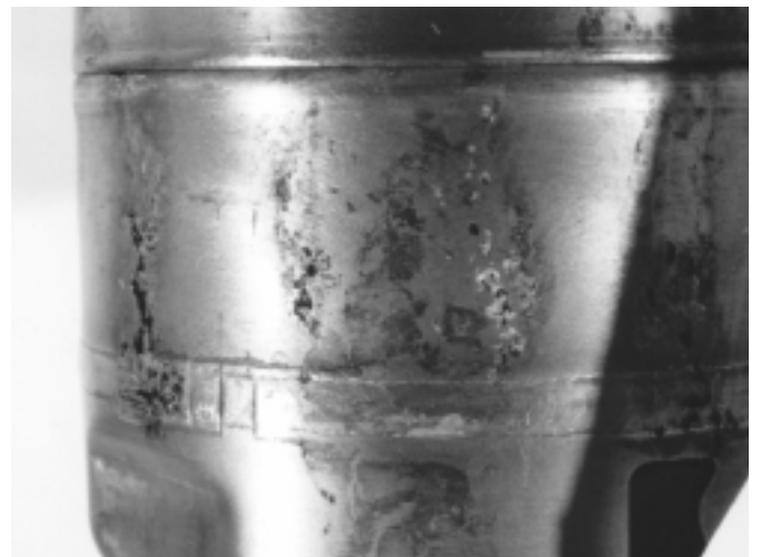
Fig. 4a: Picture showing pitting on a stainless steel component
