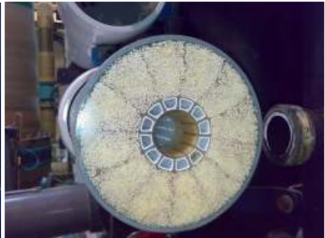
Figure 9 – UF membrane after CIP
