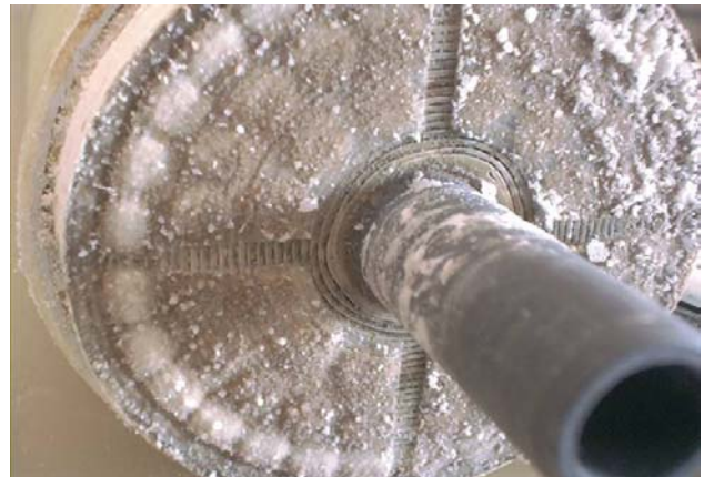
Figure 3: Calcium sulphate last stage element
