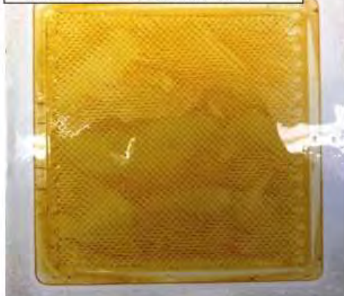
Fig 3: Blank: Fe Fouled membrane
