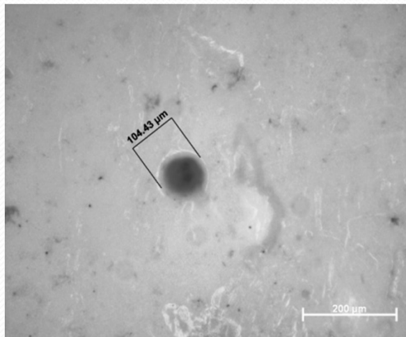
Large pinhole No. 1: 104 μm diameter
