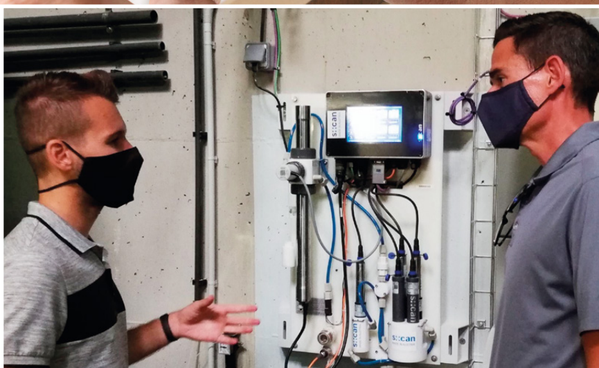
Matt Stuyvenberg (right) visits with a major metropolitan customer about their usage of s::can micro::stations which provides 15 water quality parameters, contamination alarms based on UV-VIS spectrum plus percentage of water sources, all in real time.
