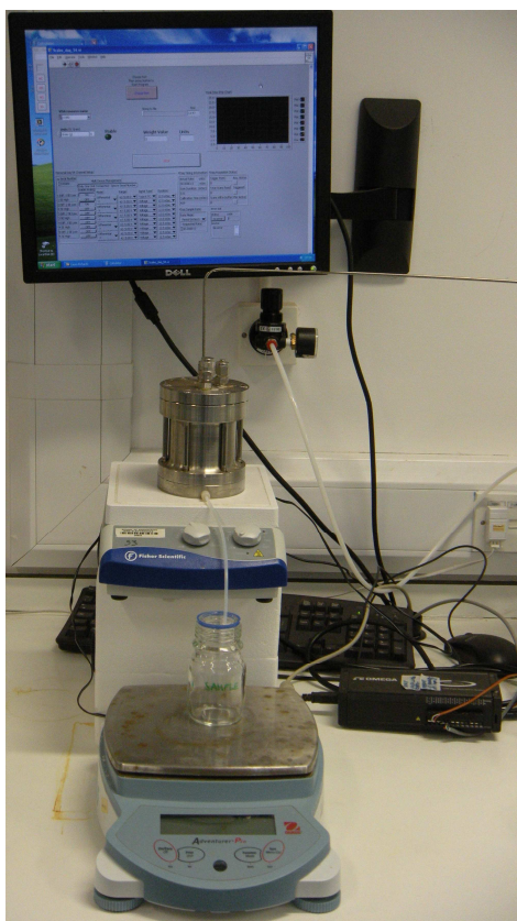
Figure 3-2. Photograph of the small stainless steel stirred cell.
