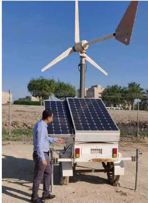
Solar PV-Wind hybrid desalination system at KFUPM
