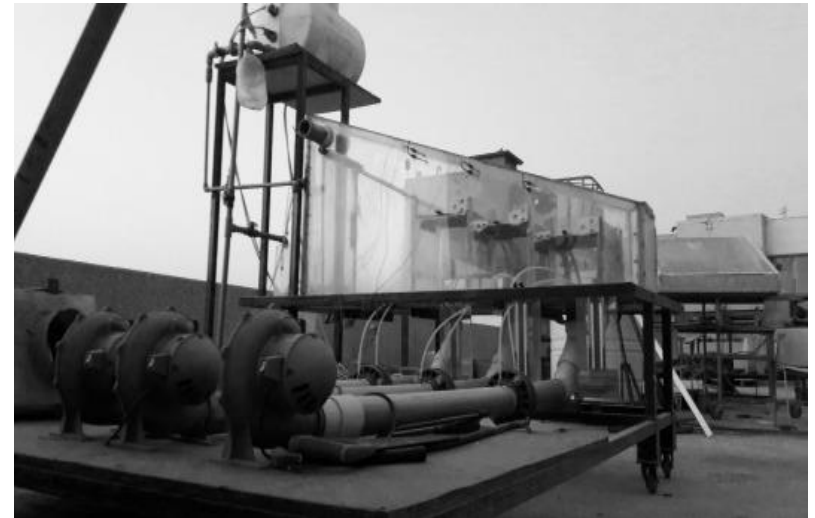
Proposed design and set up of the multistage bubble column humidifier
