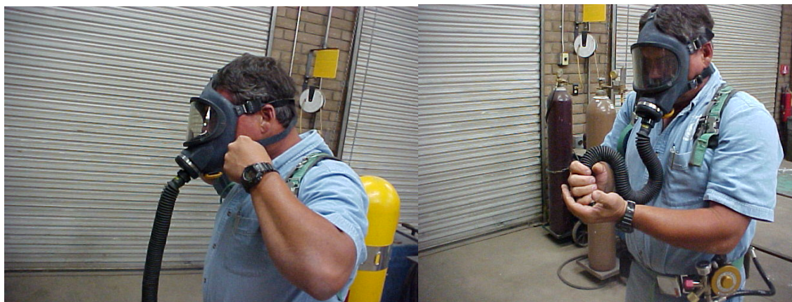
Drawing spiders tight and checking seal on facemask.
