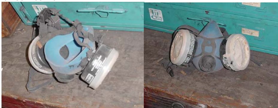
Unacceptable maintenance and storage (OSHA Violation)
