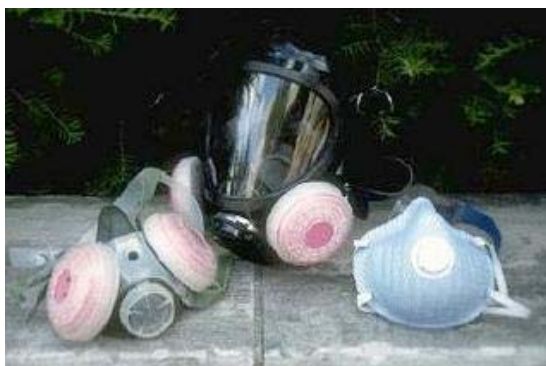
Examples of half-face and full-face respirators with HEPA filters (left and center). The mask on the right is only suitable for non-hazardous, non-respirable nuisance dusts.
