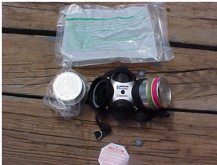
Half face type respirator with replaceable filters.
