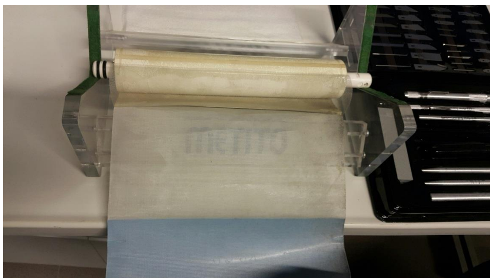
Figure 3-4: Membrane autopsy setup.
