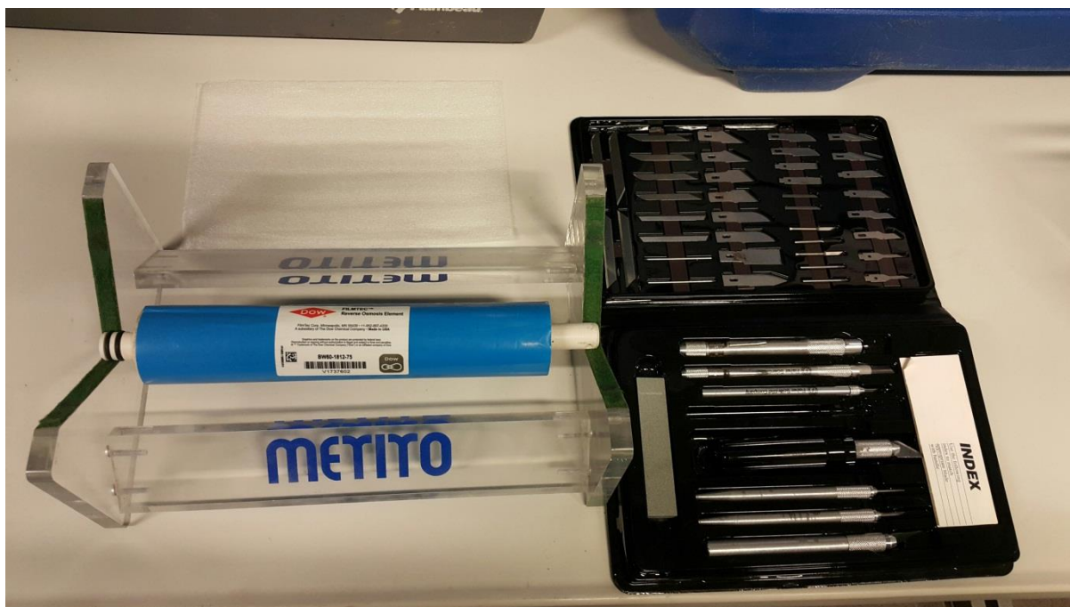
Figure 3-3: Membrane and Autopsy Preparations.
