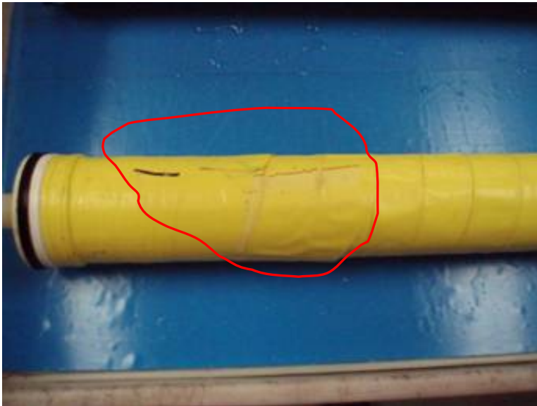
Photo 1: tape wrinkled and came loose
