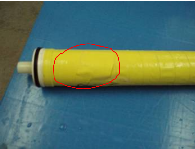
Photo 3: tape wrinkled and came loose
