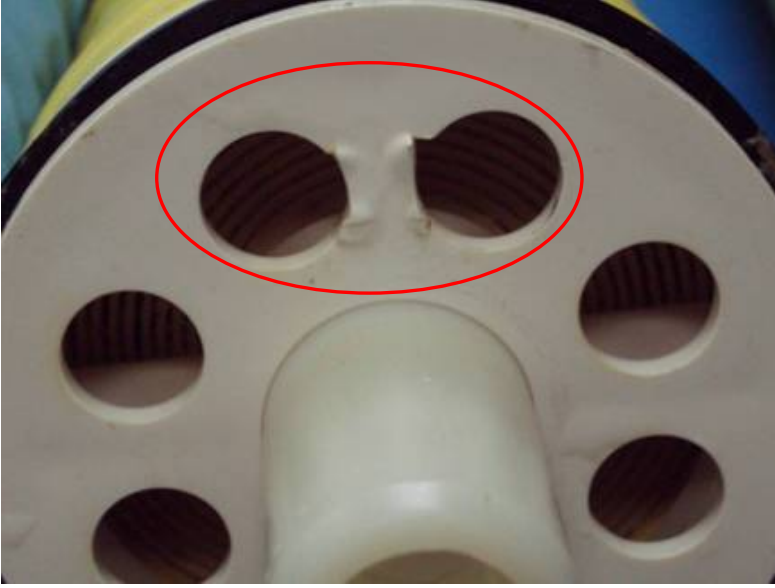
Photo 4: damaged end cap on feed end
