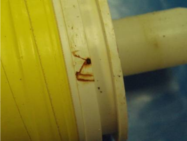
Photo 2: end cap and permeate tube on concentrate end are dirty
