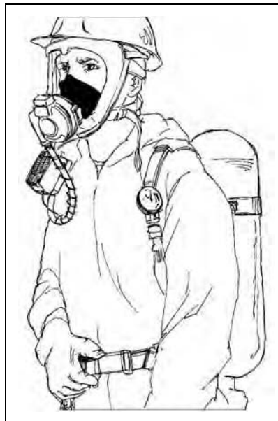
SCBA. Workers Compensation Board of British Columbia – Chlorine Safe Work Practices, 2006
