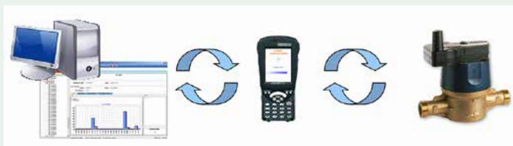
Figure 4. System Architecture: Software with data transfer to billing department (L); Meter reading device (M); water meter with radio module (R ) (Itron India, 2009).
