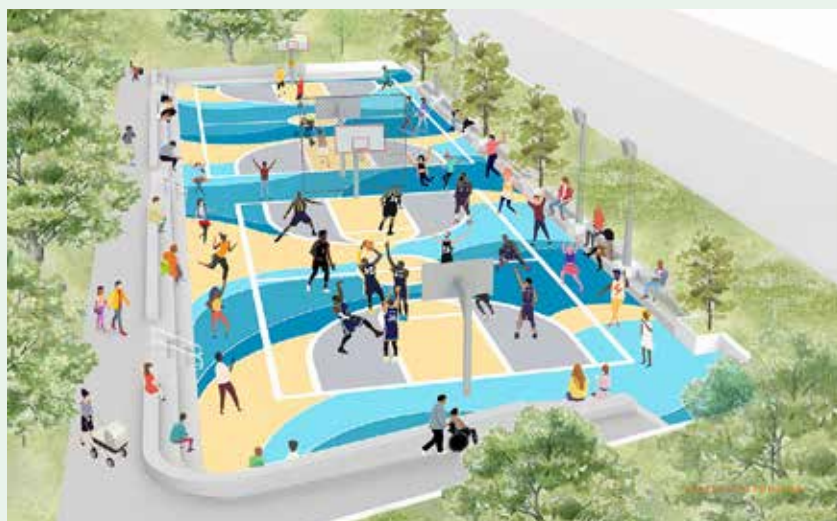
Figure 3. As part of the South Jamaica Houses cloudburst pilot project, an existing basketball court will be excavated to create underground water storage and repair the surface. The new “cloudburst” design will lower the basketball court, allowing it to fill with water during extreme rain, and will provide a new seating area for residents.
