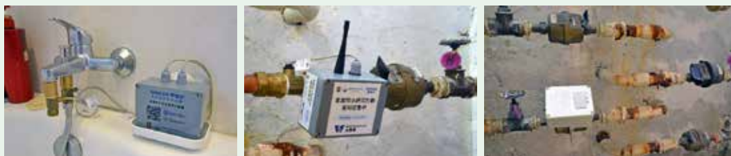
Figure 3. A Smart Tap Sensor (top-left); an in-line Smart Meter (top-right); and a Smart Meter Analyzer prototype (bottom)
