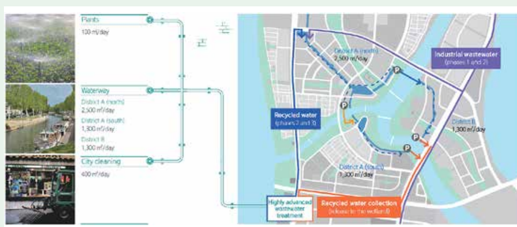
Figure 16. Water Reuse Concept Design Source: K-water (2018) 25
