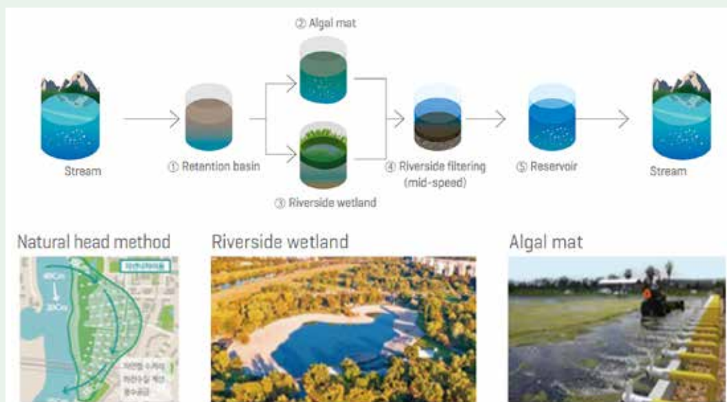
Figure 13. Eco-Filtering: Key Technology and Process Source: K-water (2018) 22
