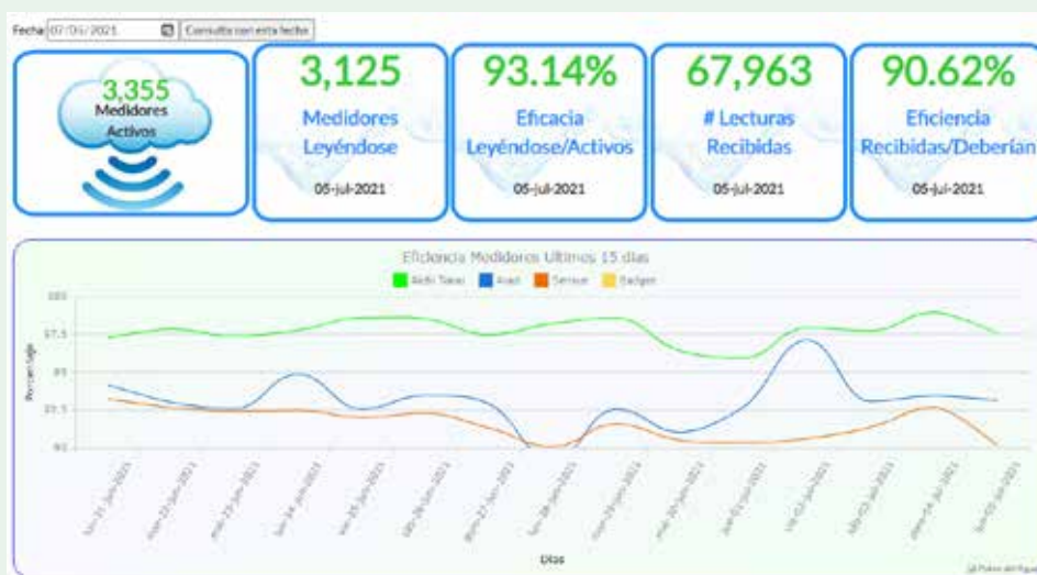
Figure 13. Effectiveness and efficiency of the several couples’Smart meters<-> Smart Network’
