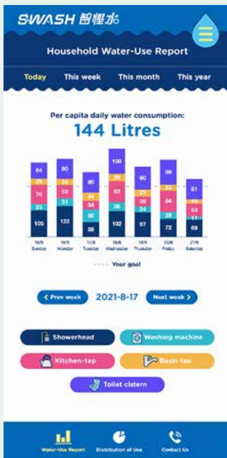
Figure 4. A mobile website for providing feedback on water use to the users
