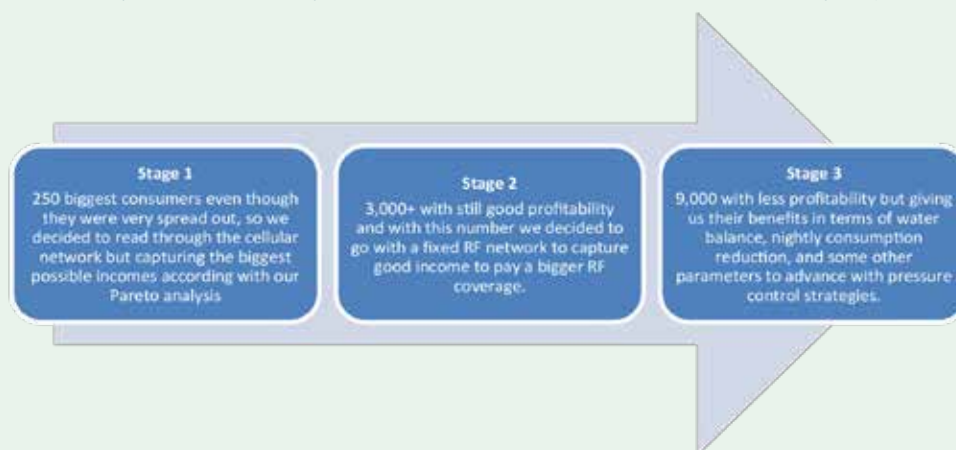
Figure 12. Three stages of the implementation of the smart metering project
