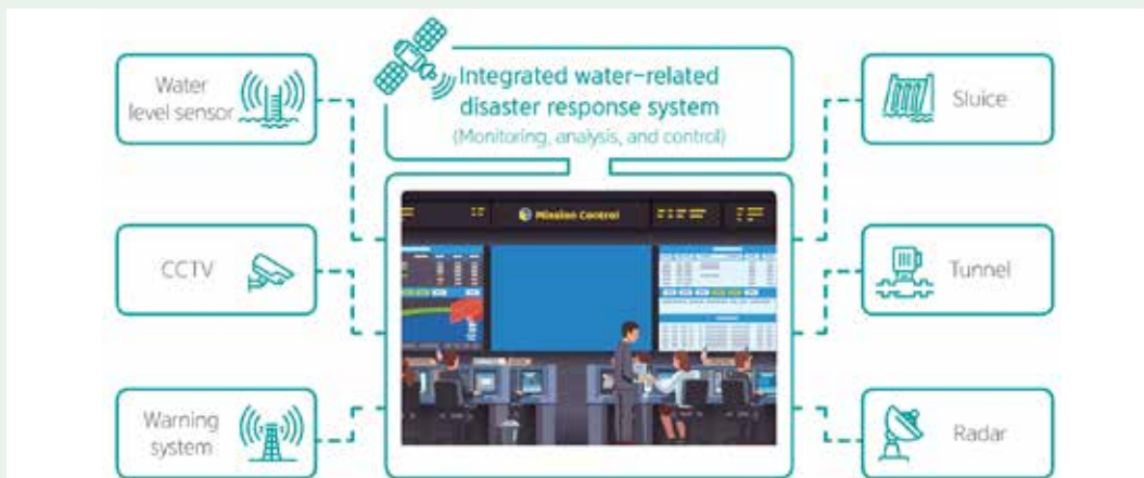
Figure 11. Integrated Water-Related Disaster Response System Source: K-water (2018) 20
