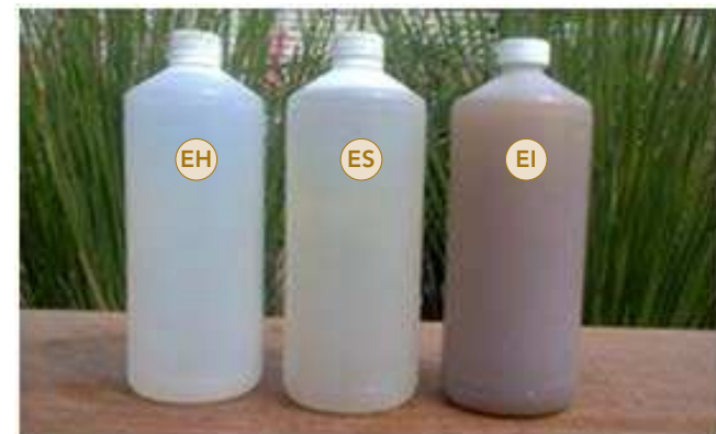
Figure 6: Observed turbidity in water sampling from inlet of the system (EI), outlet to the settler (ES) and vertical wetland outlet (EH) (Source: Alexandra Garcia)
