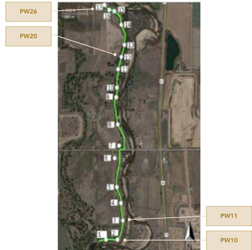
Figure 1: Aerial map of the riverbank filtration well field along South Platte River at Brighton, Colorado showing locations of sampled wells (PW: production well) (Drewes et al. 2015)
