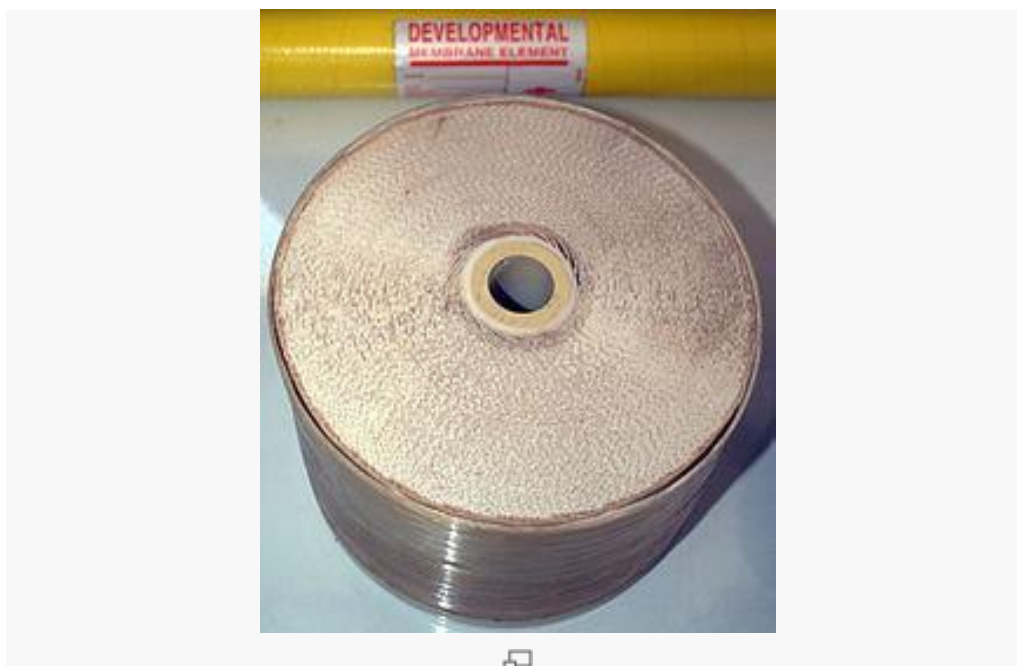
Fig. 2.2: A Semi Permeable Membrane Coil used in Desalination
