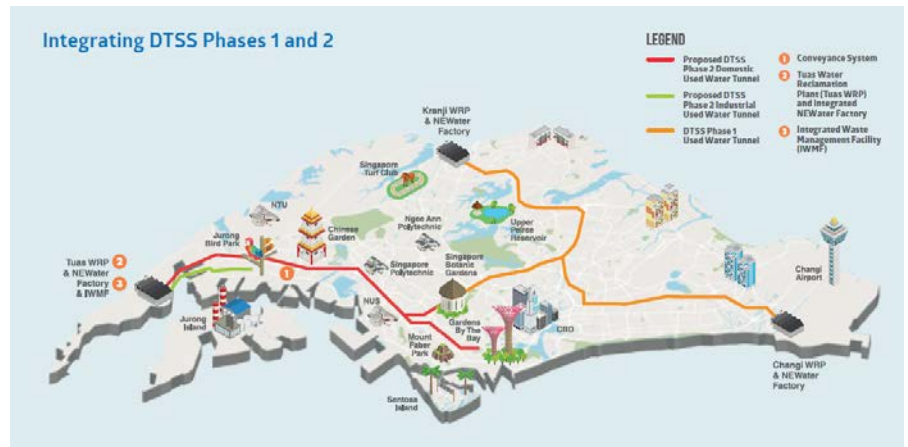
Figure 102. Used Water Superhighway – Wastewater is Being Channeled to Changi and Tuas
