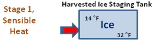
Figure 2.11, Case Study 2.1, US Units, Stage 1 Sensible Heat Calculation
