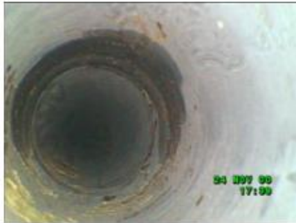
Leaking tube-to-tubesheet joint at the inlet (hot) side
