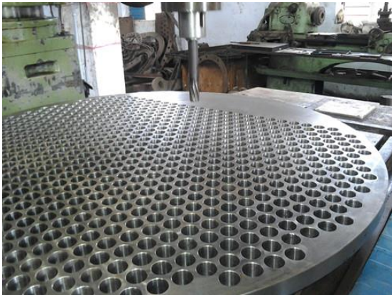
Tubesheet Hole Drilling
