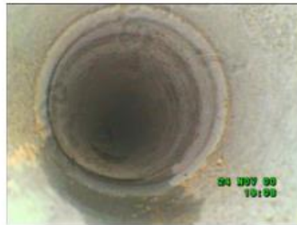
Leaking tube-to-tubesheet joint at the inlet (hot) side
