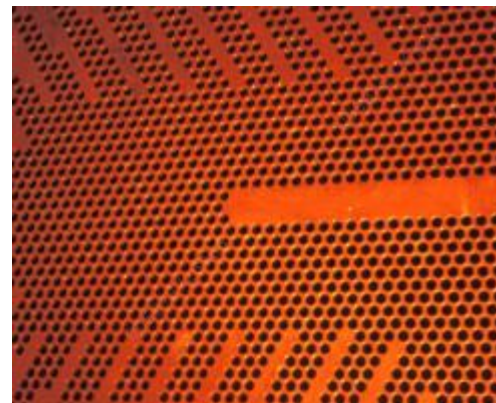
Epoxy Coated Tubesheet
