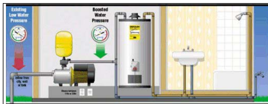
Figure 44a Typical small residential plumbing system.
