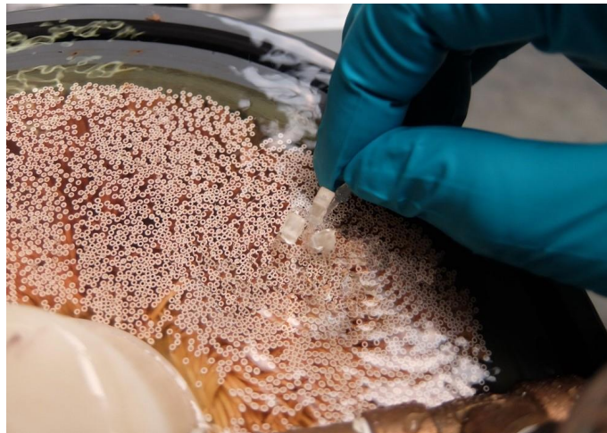
Figure 37. Identifying leaking fiber at location of large bubble
