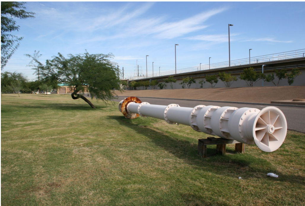
BFP – 12 inch diameter multi-bowl vertical turbine well pump.
