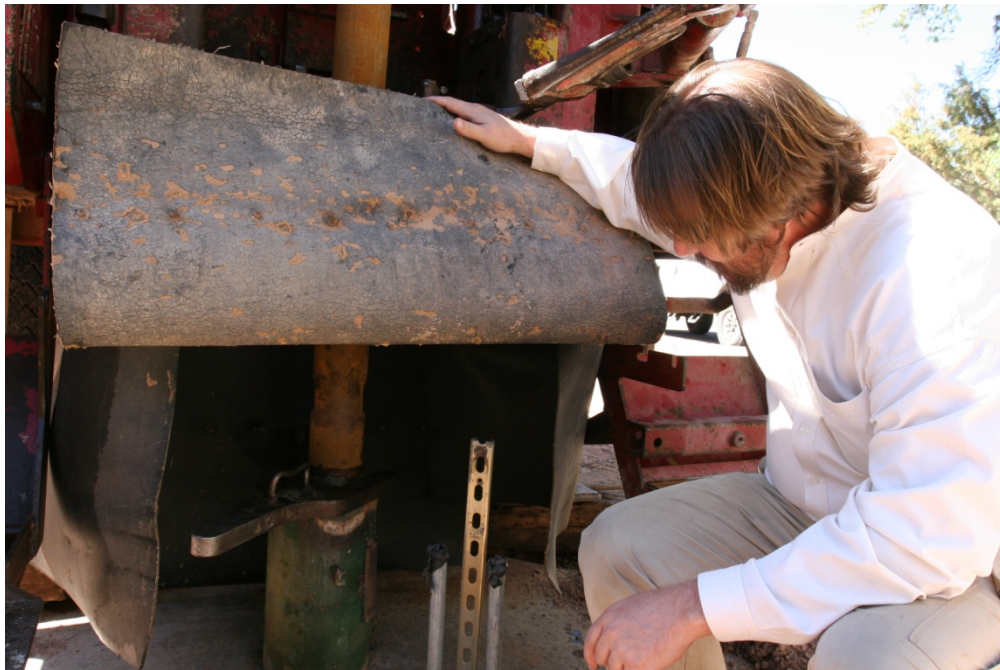
Top, drilling deck, below, well secured under drilling deck with pipe and pipe slip.
