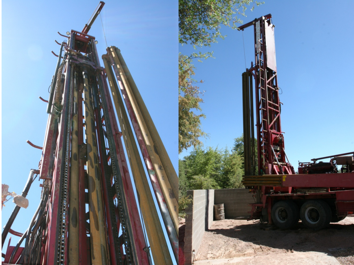
Top, drill rigging mast. Below, drilling rods on carasell and rack, notice copper pipe thread coating which prevents thread lock during high torque.
