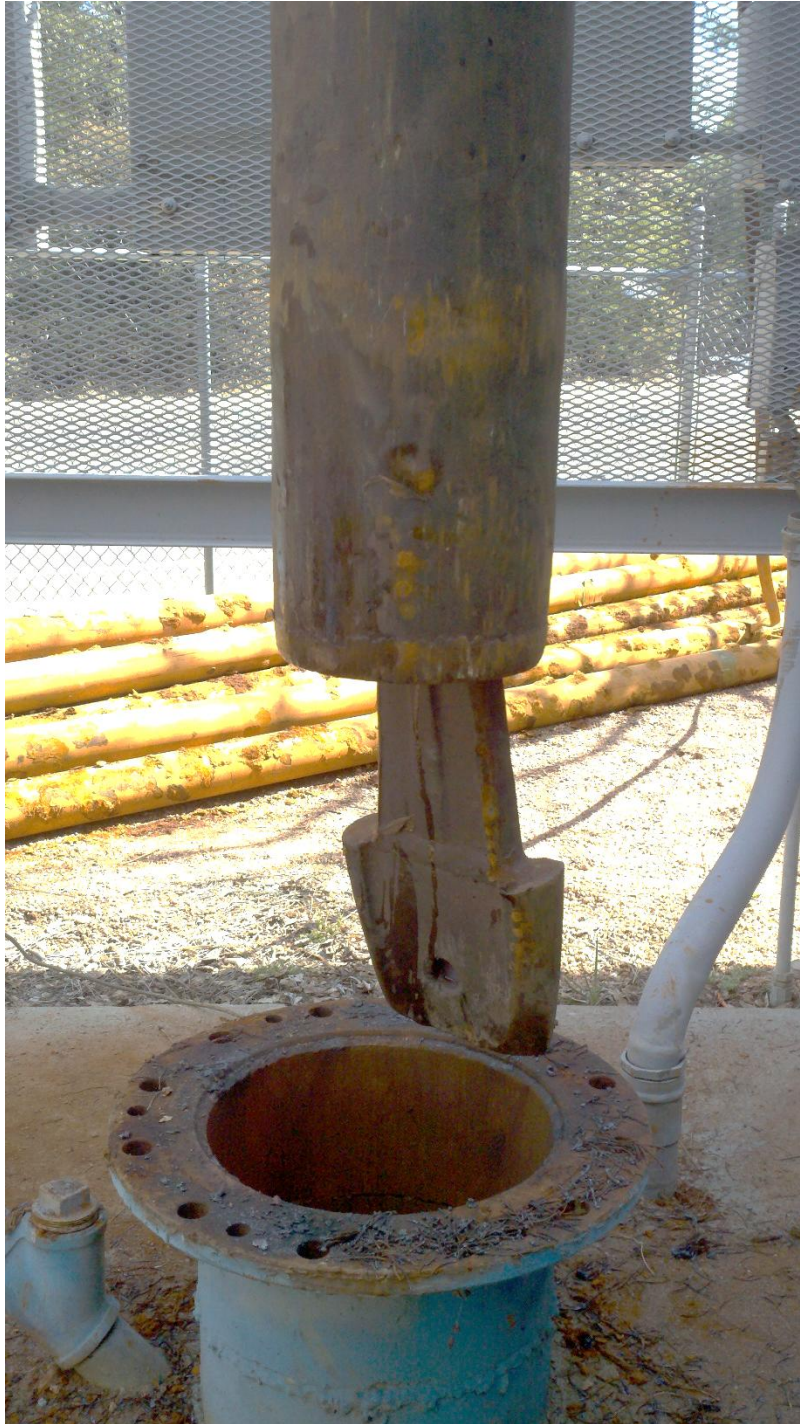
Large Bullnose Bailer Fills from the bottom up great for removing water from the casing.
