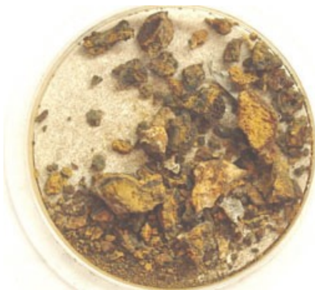
Large Rust Particles
