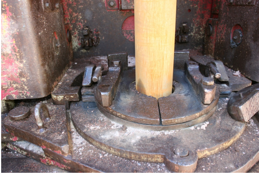
Top, drilling deck, below, well secured under drilling deck with pipe and pipe slip.
