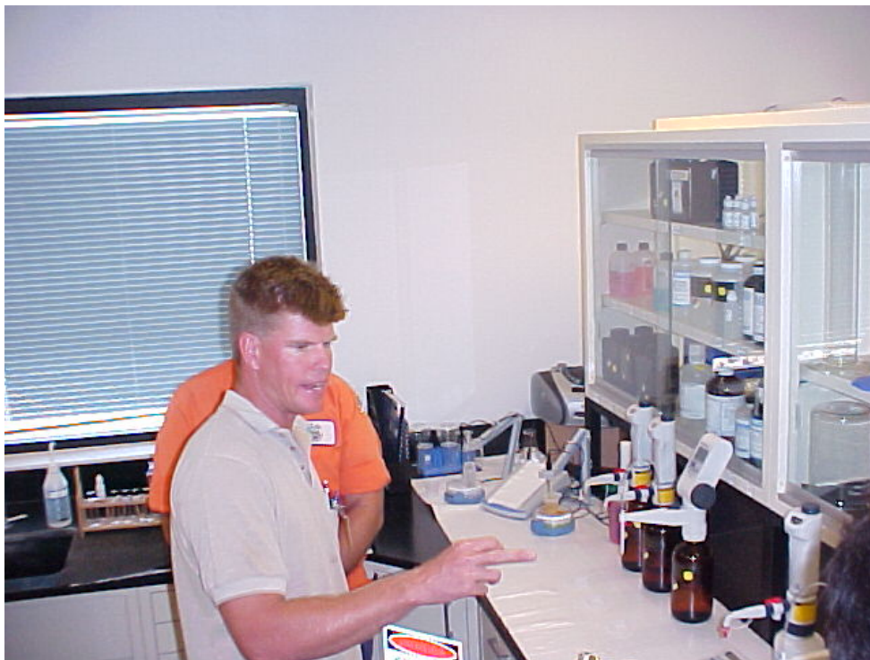
The jar test is an attempt to duplicate water treatment plant conditions.
