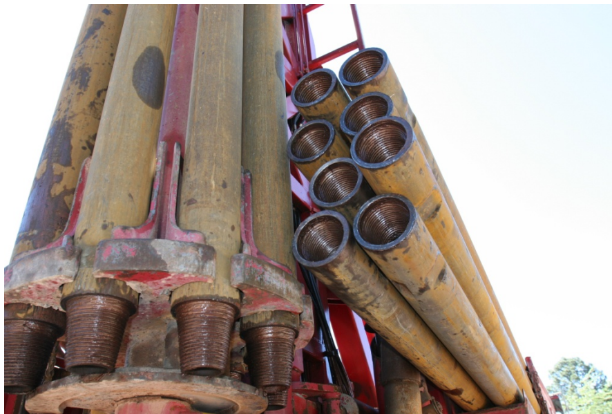
Top, drill rigging mast. Below, drilling rods on carasell and rack, notice copper pipe thread coating which prevents thread lock during high torque.
