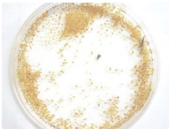
Zeolite particles from a household water softener.
