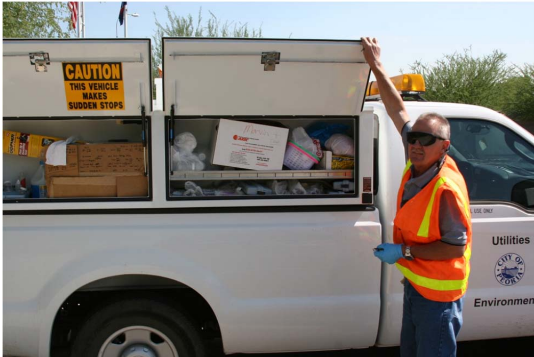
Modern water quality or sampling truck set-up. Various tools, rope, hammers are nice to have but not always necessary. I like that this sampler wears a reflective vest and gloves, I think he is safety conscience.
