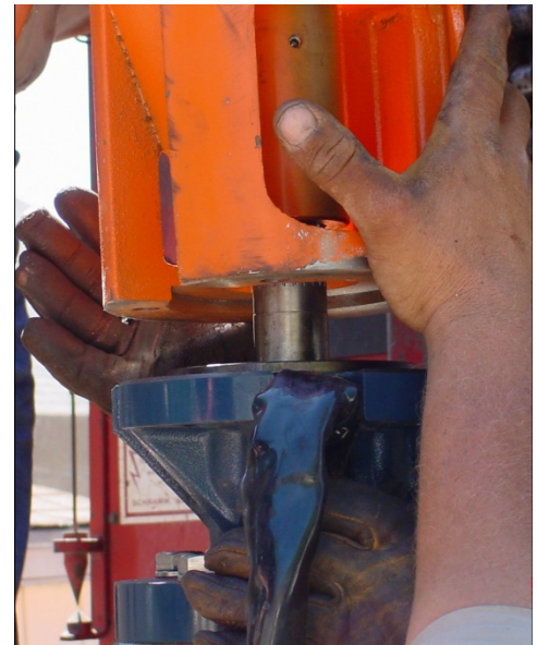
Insertion of motor spline into the pump keyway.
