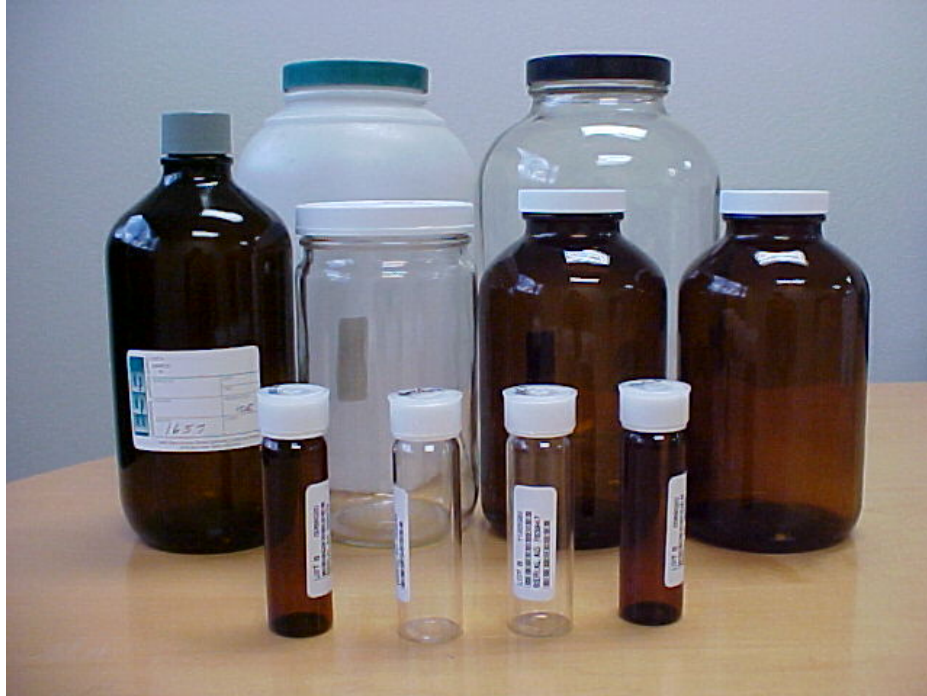
625/608, 1657, TTO/Organics, TPH/Oil/Grease, Smaller bottles-TOCs, VOCs, 601/602 and 502.2
