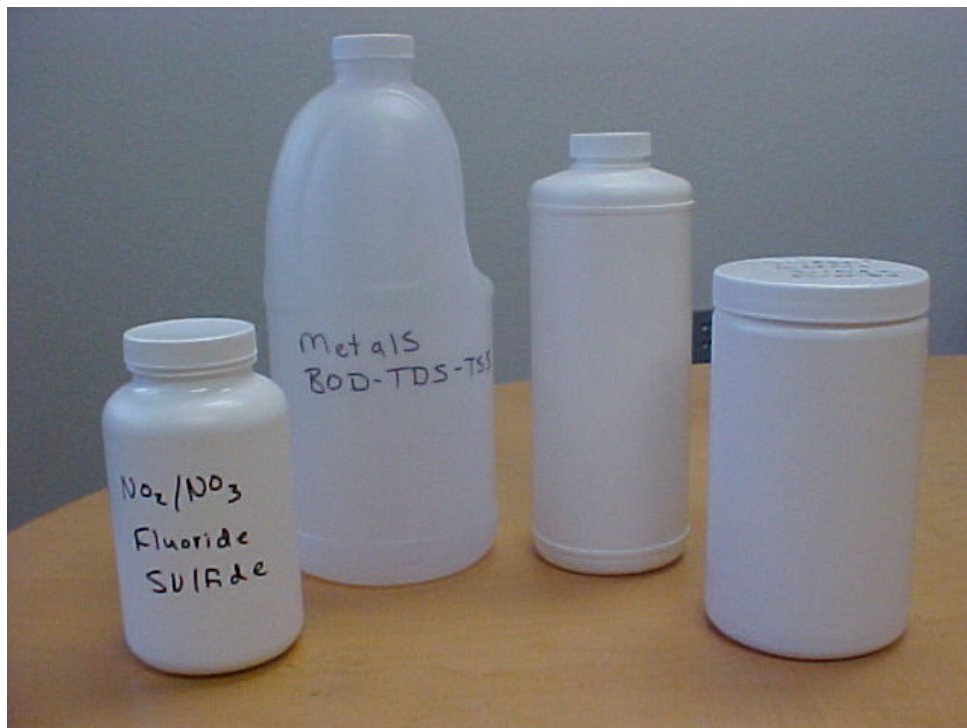
NO 2 /NO 3 , Fluoride, Sulfide, Metals, BOD-TDS-TSS Wide-mouth Sludge/Metals bottle
