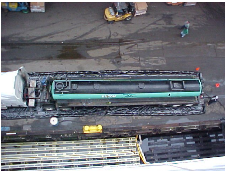
Plastic containment protection under oil tanker truck.
