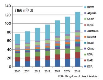
Figure 7 - Global installed desalination capacity, 2010-2016, (PikeResearch, 2010)
