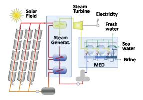
Figure 5 - CSP power plant with oil steam generator and MED desalination (Zachary et al, 2010)
