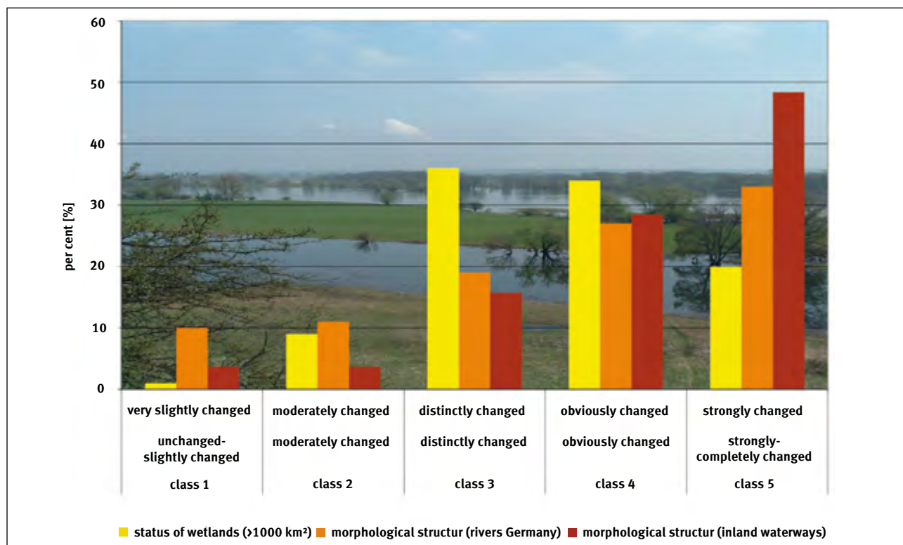
Figure 26: Distribution of floodplain status assessments (rivers with a catchment area > 1,000 km 2 ), the structural quality of watercourses (33,000 km as at 2001), and the structural quality of Federal waterways
