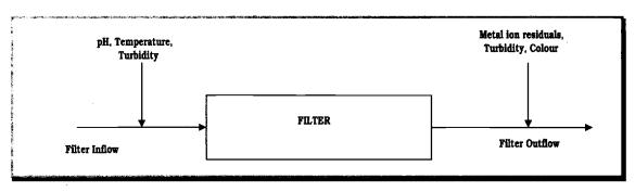
FIGURE 11: FILTRATION PROCESS MONITORING - PARAMETERS AND LOCATIONS
