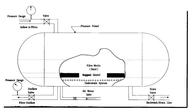
FIGURE 8: PRESSURE FILTER
