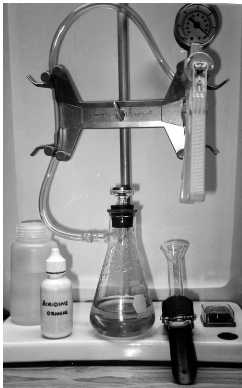
Figure A-1 Vacuum flask and pump for membrane filtration.
