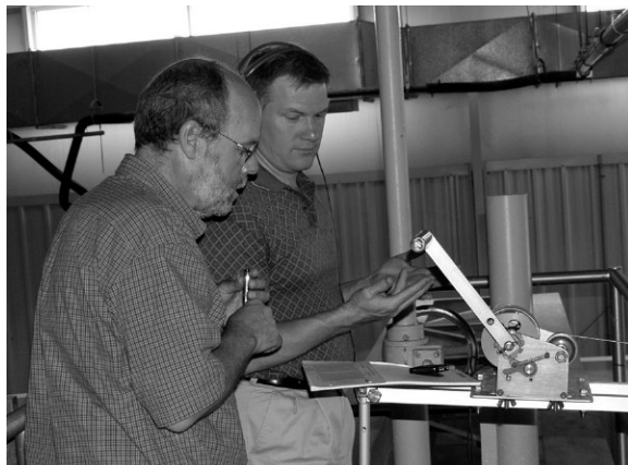
Figure 8-4 Vertical positioning of flow meter.
