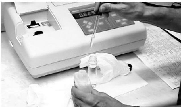
Figure C-2 Turbidity analysis—with and without acidification.
