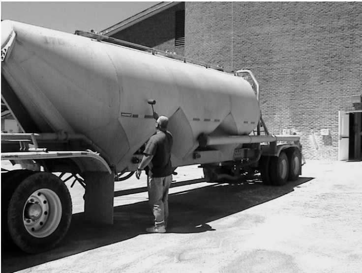
Figure C-24 Powdered lime is pneumatically transferred into building-enclosed hoppers from a hopper-bottomed truck.
