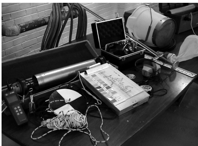
Figure 10-10 Lake water sampling equipment.
