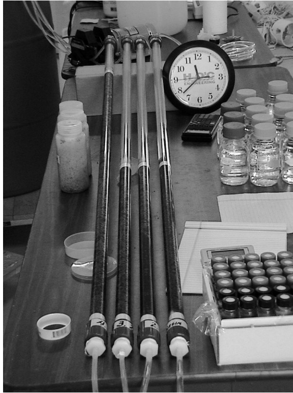
Figure 12-1 Experimental set-up of GAC test columns.
