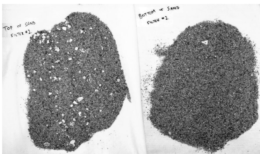
Figure 5-23 Appearance of sand removed from top and bottom of layer.
