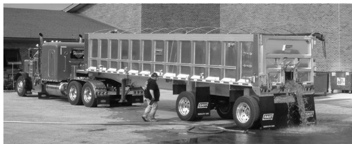
Figure 5-16 Recovery of used GAC in trailer.
