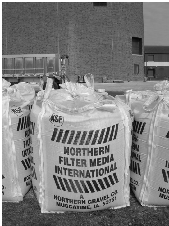
Figure 5-17 Filter sand in totes.
