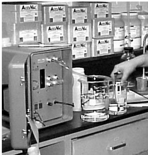
Figure 4-2 Particle enumeration and sizing using an electronic particle counter.
