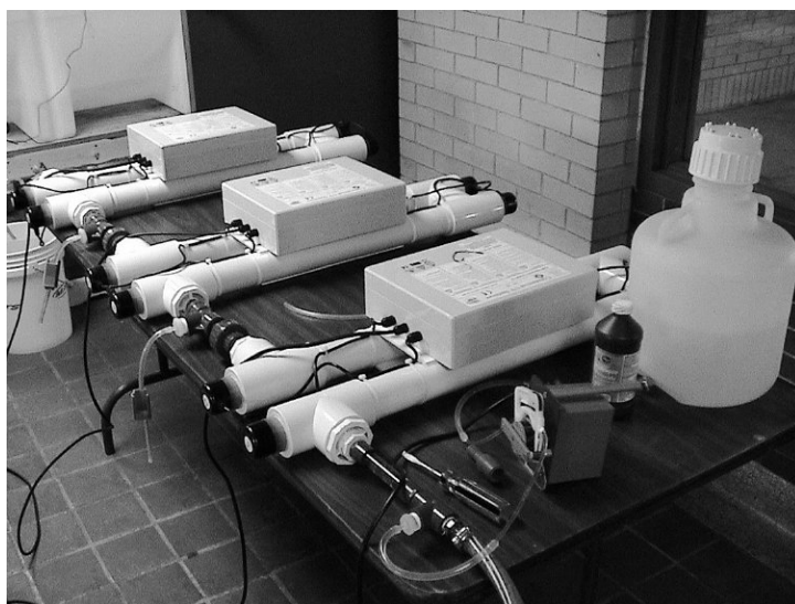
Figure 12-19 Ultraviolet light test apparatus.
