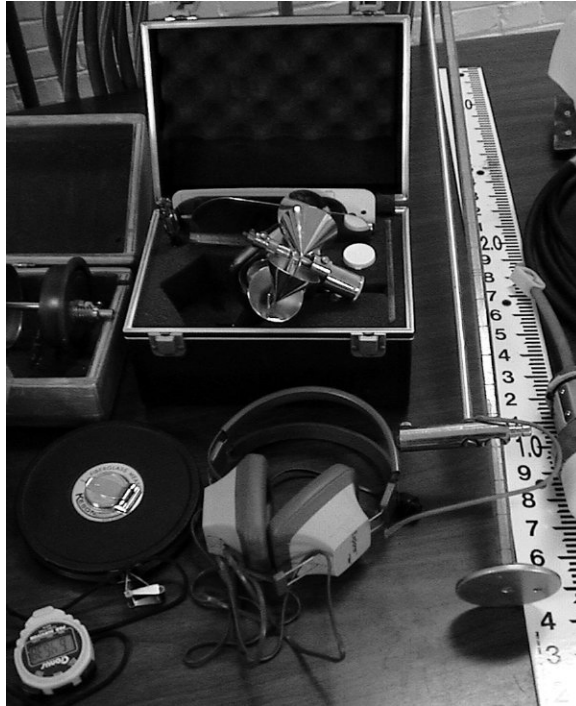
Figure 10-11 Stream flow and depth measurement apparatus.
