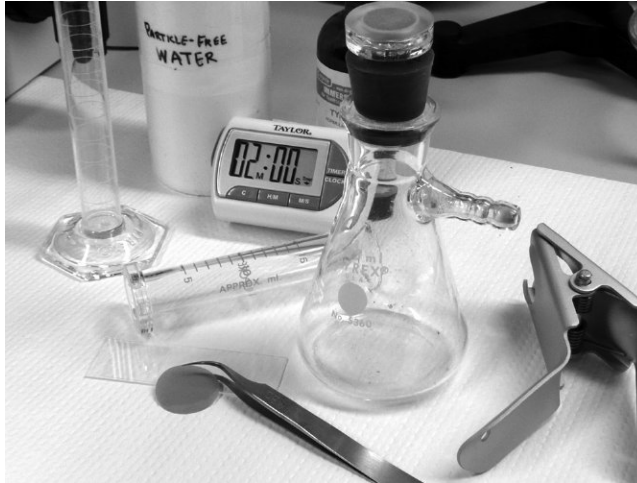
Figure A-2 Membrane filter apparatus, forceps, microscope slide, timer, particle-free rinse water.
