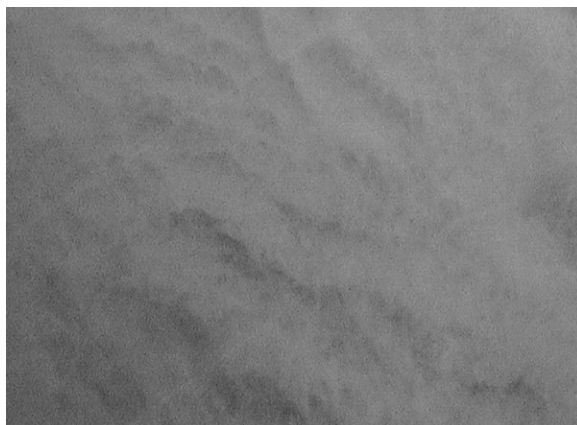
Figure 8-5 Smooth striated surface indicates spiral flow.
