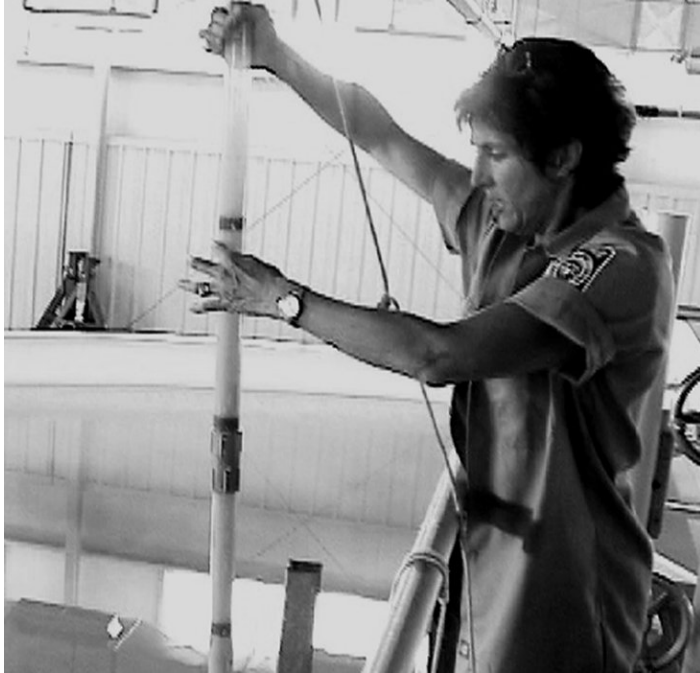
Figure C-20 All softeners require effluent sampling plus checks of lime feed valves, flow rates, and stability of slurry blankets.
