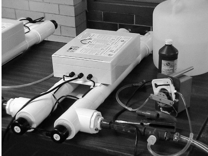
Figure 12-20 UV-catalyzed hydrogen peroxide oxidation of organic matter.
