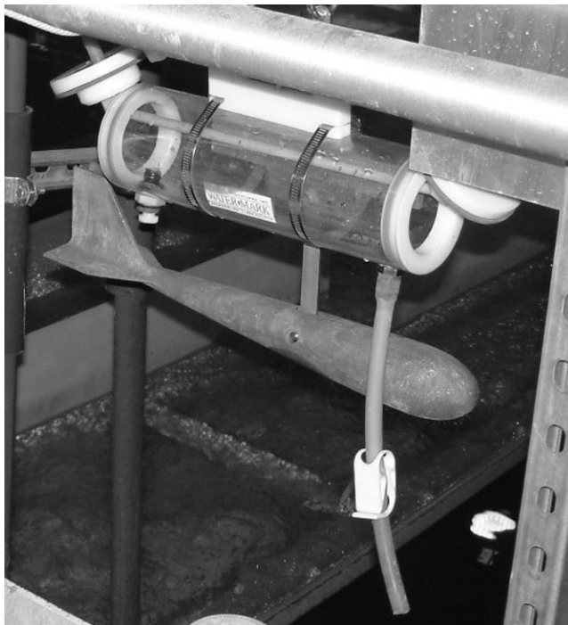
Figure 6-4 Slurry blanket sampling device.
