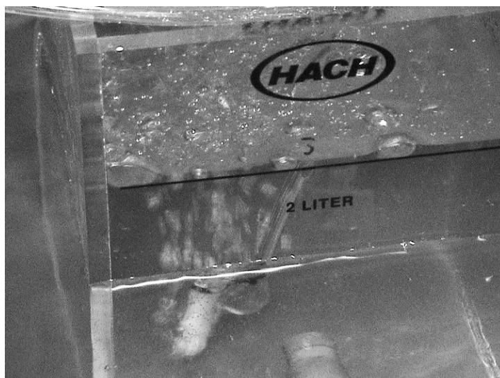
Figure 11-7 Incomplete odor reduction by aeration.
