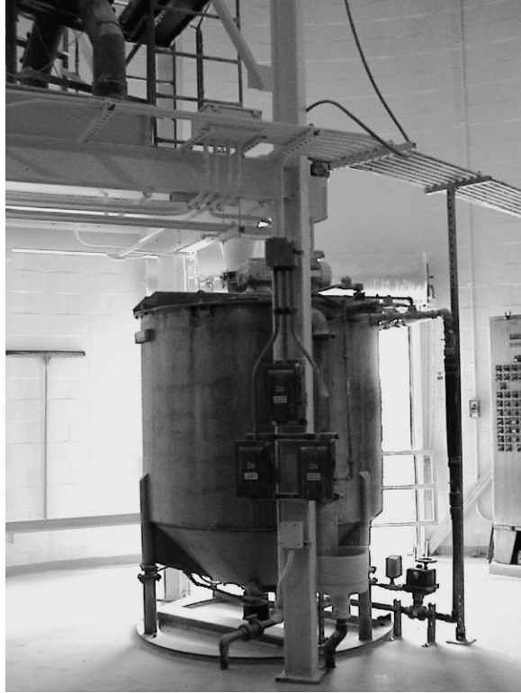
Figure C-27 Batch-process lime slaker.
