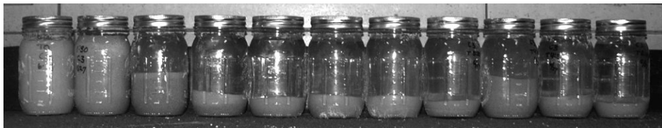
Figure 6-12 Grit removed during revised gritting procedure.
