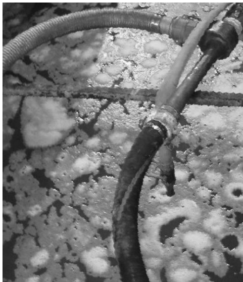
Figure 5-9 Air bubble release causes foaming.
