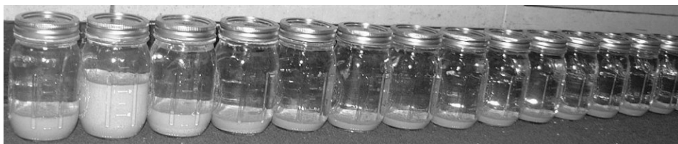
Figure 6-10 Grit removed over 5 minute gritting period.
