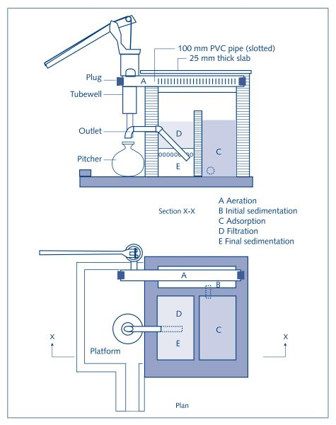
Fig. 13.2. Hand-operated aeration/filtration unit
