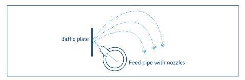
Fig. 13.6. Simple spray aerator using baffle plate
