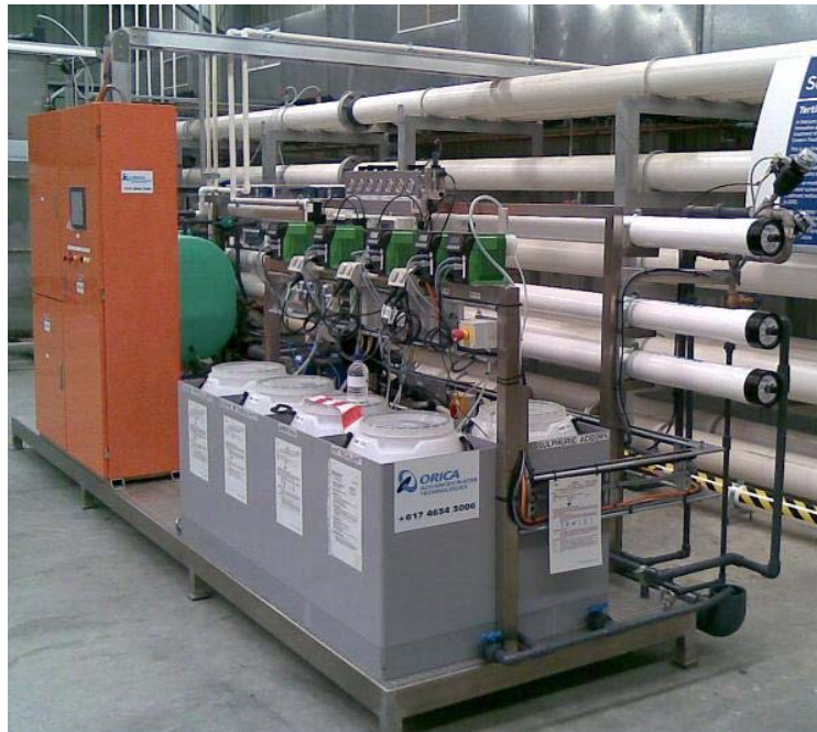
Above. Reverse Osmosis Plant, with pre-treatment
