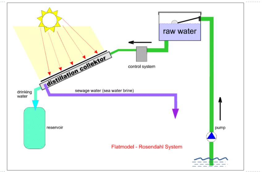
In the aforementioned stills, the distance between the brine surface and the clear inclined glass plate tends to become smaller from (1-4 in) in an effort to **minimize heat loss** through convection currents in the space between the brine surface and the inclined glass cover, which assists in *increasing the* efficiency of the still, i.e., the productivity (fresh water in L/d).
