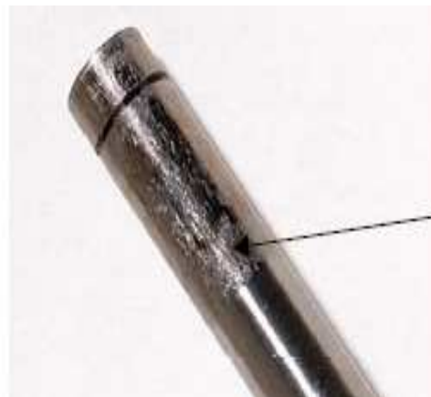
Plunger scuffing due to excess water
