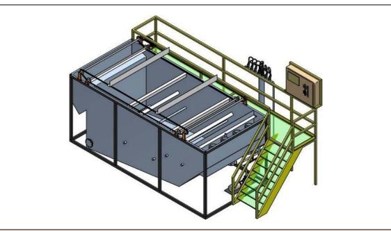
Figure 1 General sketch of square flotation chamber with a system of surface skimmers.
