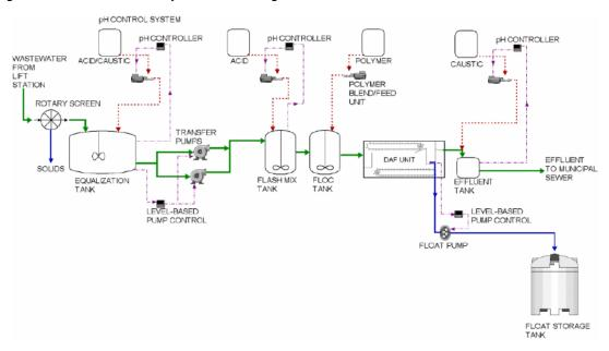
Figure 13.- Integration of a DAF system in a WWTP pretreatment (Ross, C., Valentine, GE et al.; 2013).
