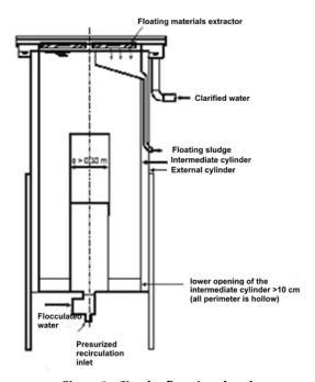
Figure 8.- Circular flotation chamber.
