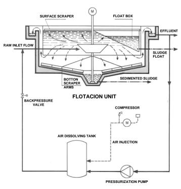
Figure 5.- Functional diagram of a circular DAF system.
