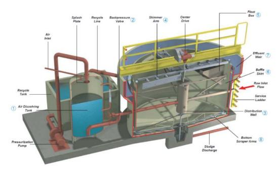
Figure 10.- Elements of a DAF system with a circular flotation chamber (ADVANCED ENERGY SOLUTIONS SAE LTDA.).
