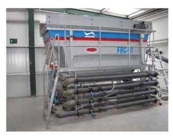
Figure 14.- DAF system with prior flocculator tube (Float Anaconda® FRC-20; 20 m3 / h; TORO).
