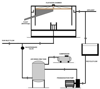
Figure 4.- DAF with recirculated flow pressurization (CEPIS, 1992)
