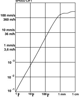
Figure 1.- Vertical speed of air bubbles as a function of diameter.
