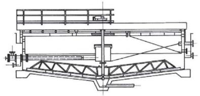
Figure 9.- Circular flotation tank floor scheme
