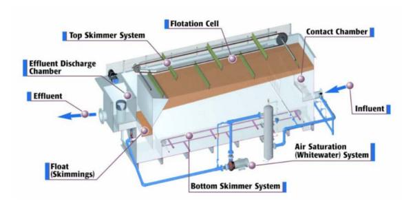
Figure 12.- Elements of a DAF system with rectangular flotation chamber (Ross, C., Valentine, GE et al.; 2013).
