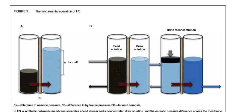
facilitates diffusion of water through the membrane (A). The FO process can be coupled with a brine reconcentration system (e.g., reverse osmosis) (B),
