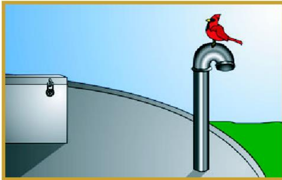
Figure 2: Storage reservoir with shoebox lid and vent
