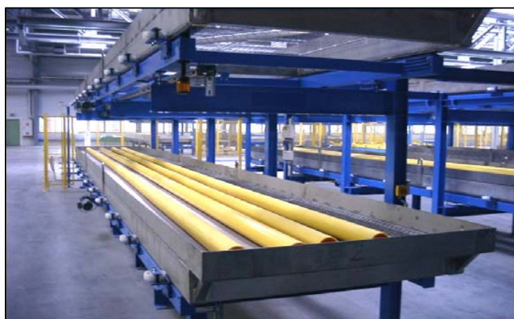
Figure 110. 12 Meter PE Pipe for EB Crosslinking
