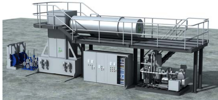
Figure 28. Easy-e-Beam 800 keV, 100 mA
