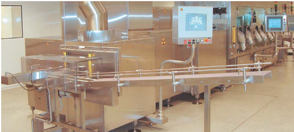
Figure 108. STERSTAR™ System for In-line EB Surface Decontamination
