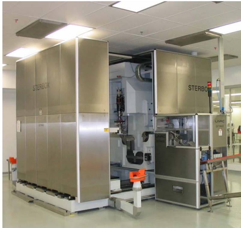
Figure 104. Self-shielded In-line Medium Energy System for Device Sterilization with Mobile Section (stainless steel housing and lead shielding) Open
