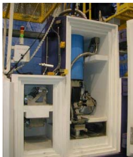
Figure 76. Self-shielded 500 keV Electron Beam for Shrinkable Film
