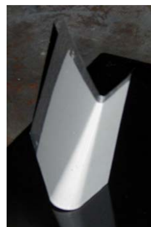
Figure 87. EB Coating after Mandrel Bend Test
