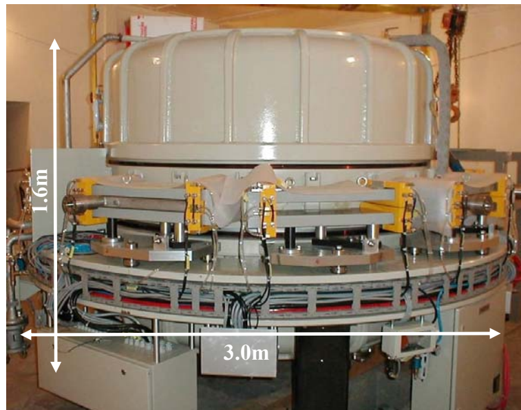
Figure 21. 10 MeV, 200 kW Rhodotron
