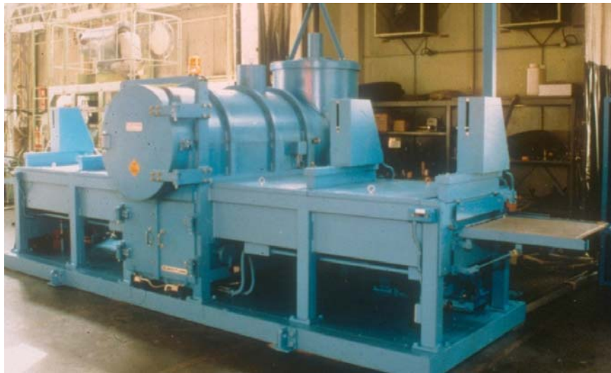
Figure 33. 300 keV, 100 mA NHV Curetron for Surface Curing on Flat Substrates
