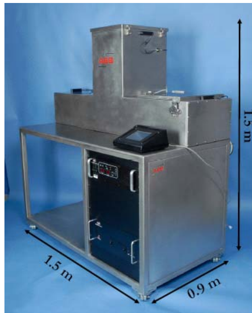
Figure 39. Self-shielded Low-energy Applications Development Unit
