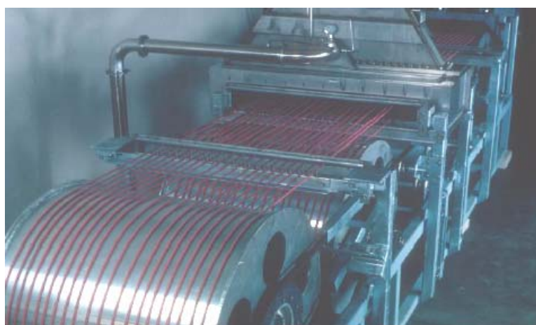
Figure 71. Wire and Cable Under-beam Transport System
