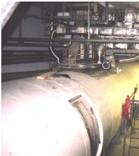
Figure 113. Flue Gas Irradiation Chamber with EB Unit
