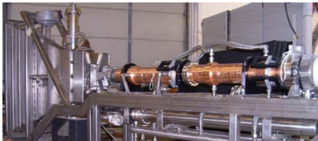
Figure 17. 30 kW 10 MeV Mevex Linac
