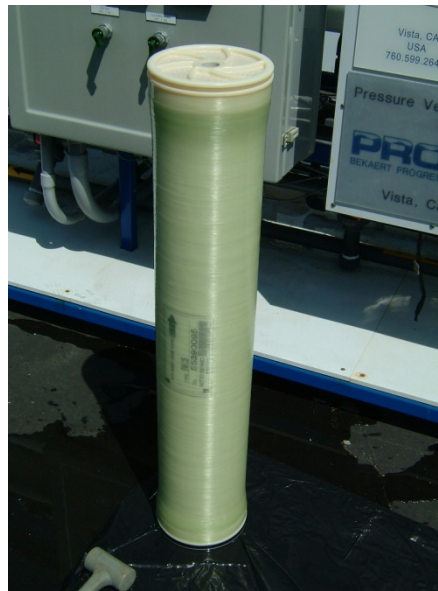
Figure 19 – Typical 8-inch Membrane Element
