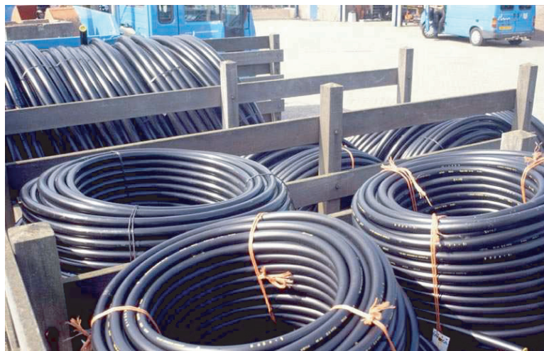
Figure 4.42. Stock of coiled PE pipes.
