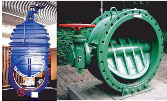
Figure 4.50. Large gate- and butterfly valves.
