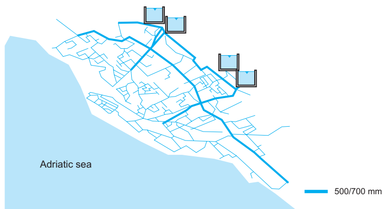
Figure 4.5. Layout of distribution network of Zadar, Croatia (Gabrić, 1997).
