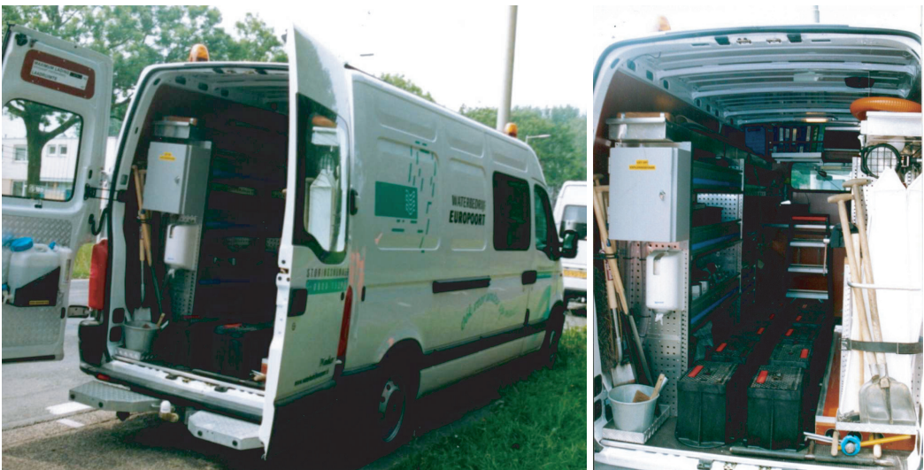
Figure 6.44. Mobile workshop for quick repair service.
